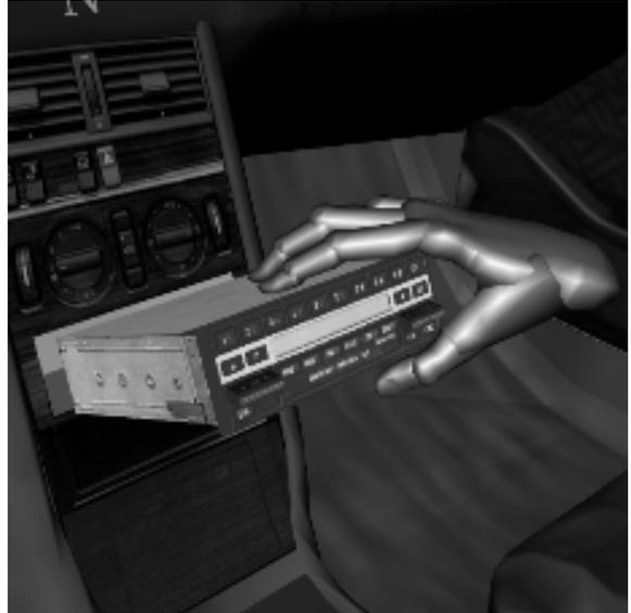
Figure 3: Ergonomy study and assembly simulation in a virtual car interior. The user has to install the car radio.
