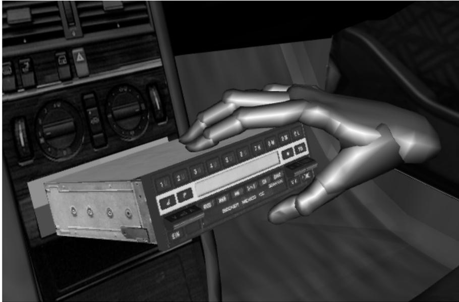
Figure 3: Ergonomy study and assembly simulation in a virtual car interior. The user has to install the car radio.
